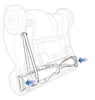
Center Belt on motor-driven shaft; test Brush Roll for easy turning.
